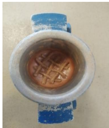
Fig. 2. Specimen preparation with one-layer of geotextile
