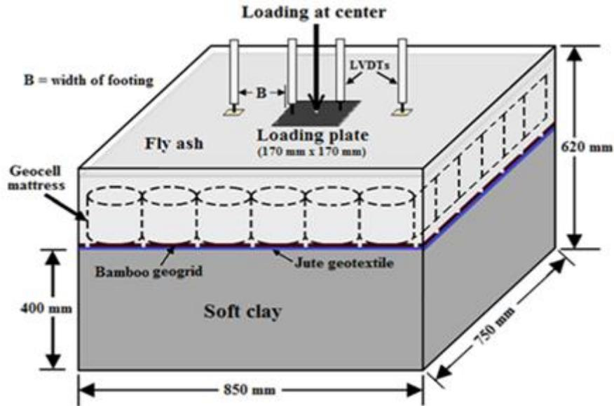
Fig. 5. Schematic of the test set up.
