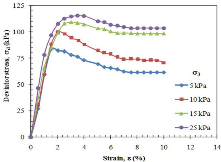
Fig.3. Deviator stress-axial strain curves of fly ash from consolidated drained (CD) triaxial tests.
