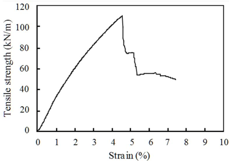
**Fig.1.** Tensile strength-strain response of bamboo geogrid.
