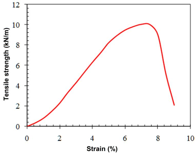
**Fig.2.** Tensile strength-strain curve of jute geotextile.
