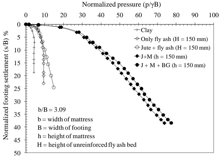
**Fig. 8.** Variation in footing pressure over geocell mattress without and with basal bamboo grid
