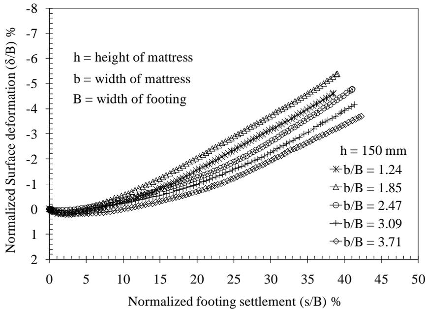
Fig. 10. Surface deformation surrounding the loaded area with varying mattress widths
