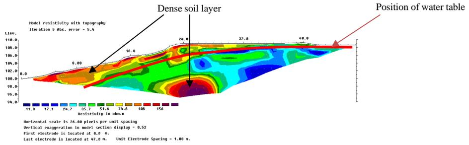
Fig.9. ERT 3, location – 3 - Along the slope (Dipole – Dipole)
