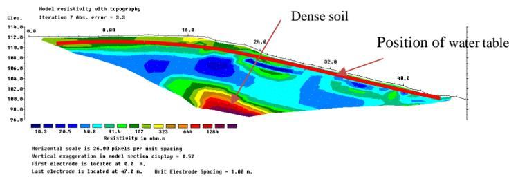
Fig.8. ERT 2, location 2 - Along the slope (Dipole – Dipole)
