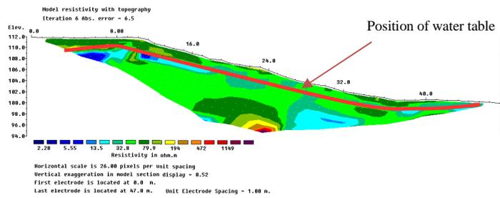
Fig.7. ERT 1, Location 1 - Along the slope (Dipole – Dipole)
