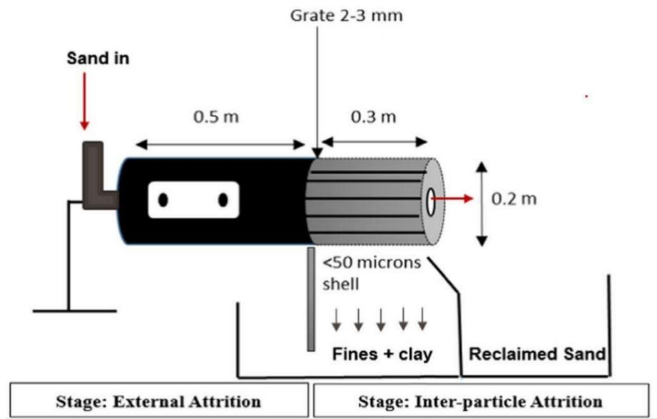
Fig 2. Reclamation device for spent foundry sand [8]
