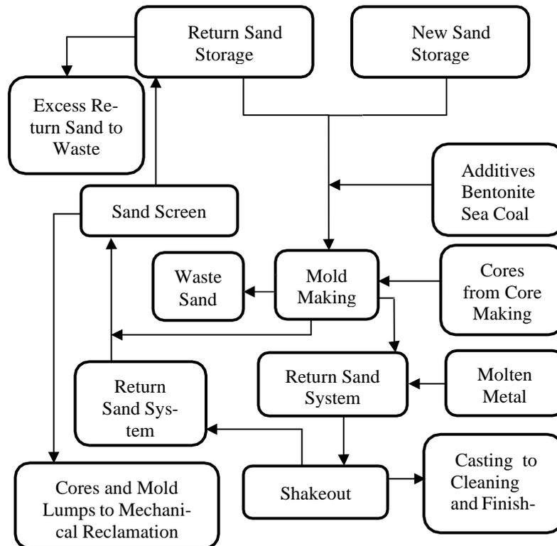
**Fig 1.** A schematic of the flow of sands through a typical foundry, [3,4]
