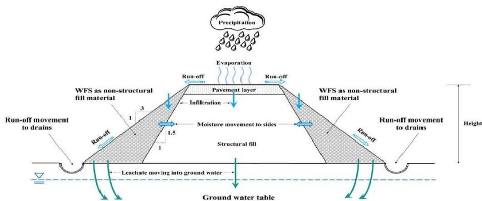
Fig 2. Water flow balance chart for WFS as fill material in road embankments [19]
