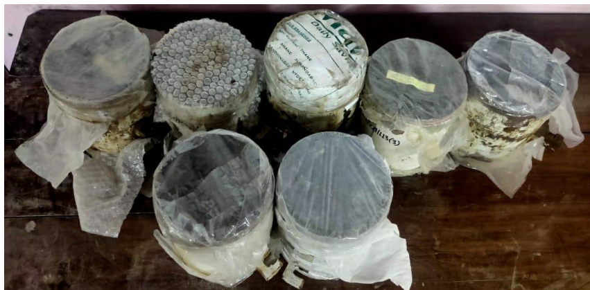
Fig. 4. Sealed Bio-Enzyme Stabilized CBR Soil Samples
