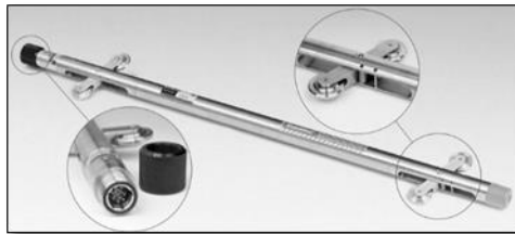
Fig. 4. Slope Inclinometer (After Kyowa Elect. Instruments)
