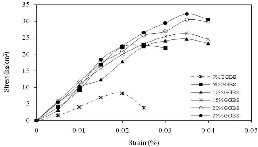
Fig. 1. Stress strain behavior of untreated clay and GGBS based geopolymer clays
