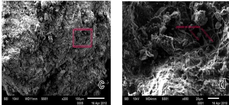
Fig. 2. SEM micrographs of GGBS geopolymer clay blends with varying GGBS content: a) 0% GGBS, b) 15% GGBS c) 20% GGBS d) 25% GGBS
