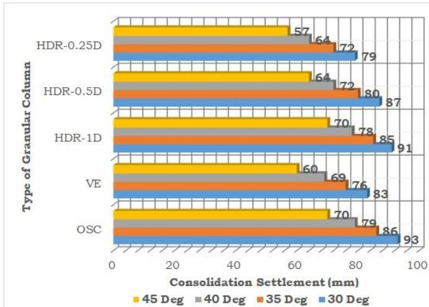
Fig.7 Effect of the friction angle of the infill soil on consolidation settlements.
