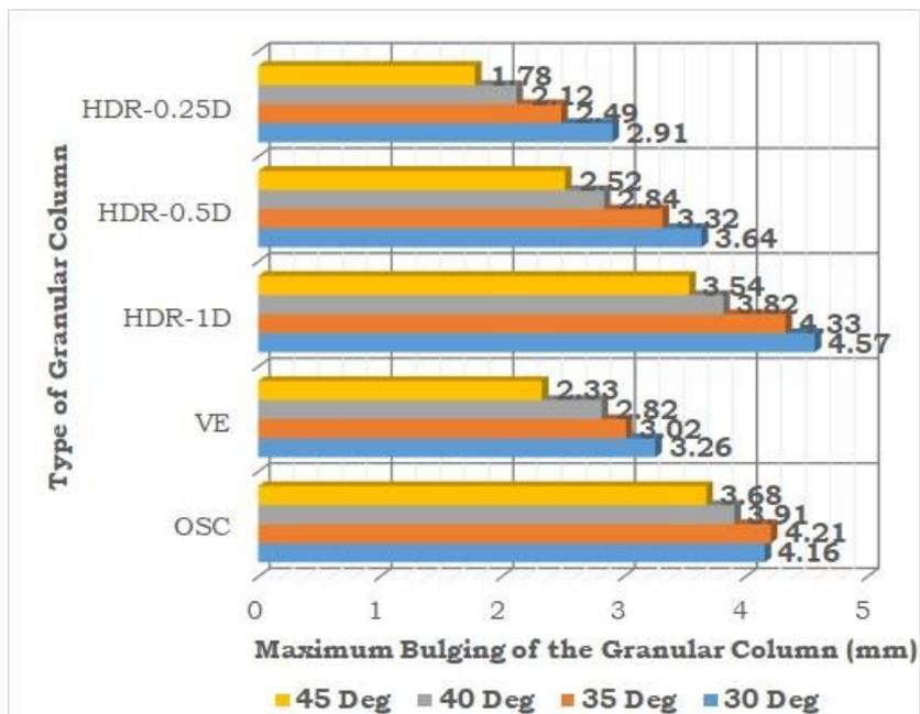
Fig. 8 Effect of the friction angle of the infill soil on bulging of granular columns.
