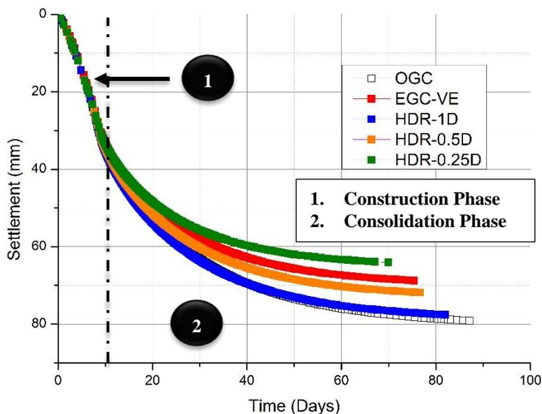
Fig. 3 Variation of settlement with time for granular columns
