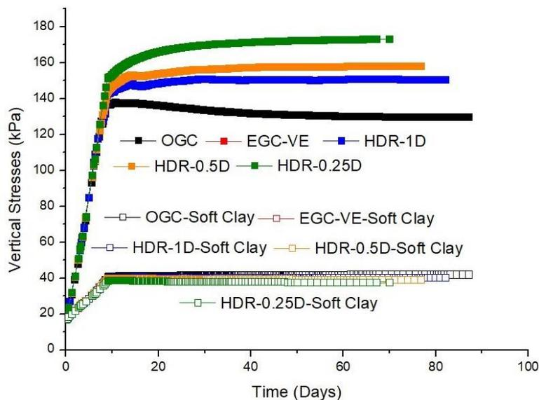
Fig. 5 Variation of vertical stresses on the granular columns and soft clay with time
