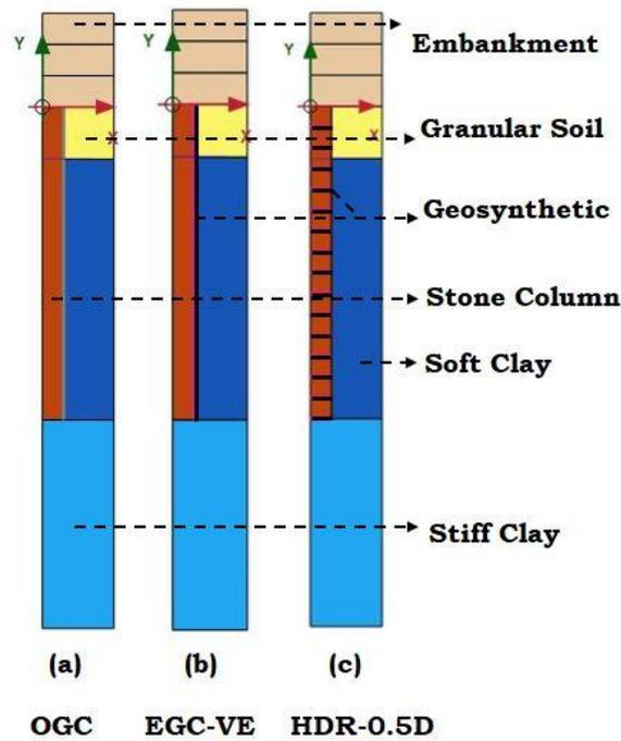
**Fig. 1** Unit cell FE models of embankments supported by ordinary and encased stone columns; VE – Vertical Encasement and HDR –Horizontal Disc Type Reinforcement.
