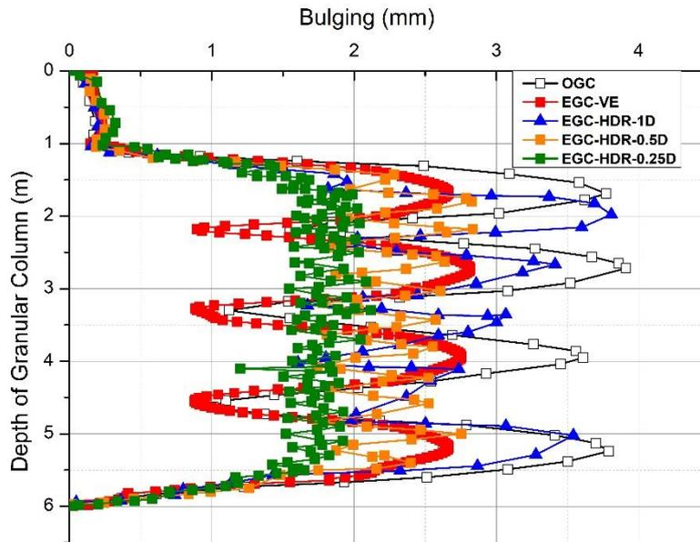
Fig. 6 Variation of bulging of the granular columns with depth
