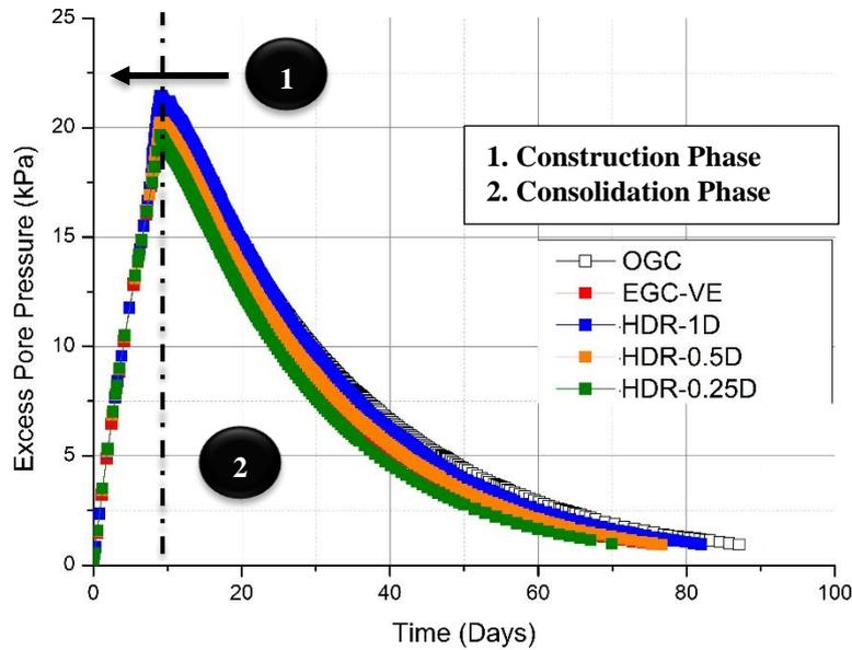
Fig. 4 Variation of excess pore pressure with time
