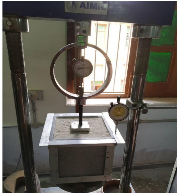
Fig. 3. Plate load test setup
