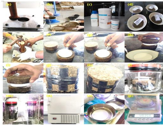
Fig. 2. Sequential sample preparation and filter paper test methodology.
