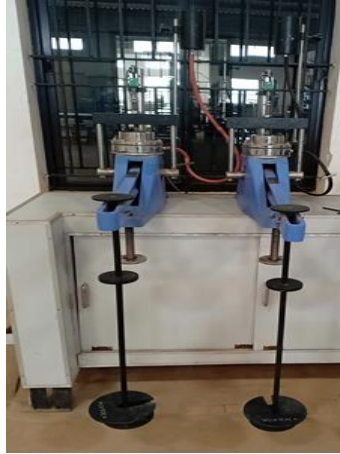
Fig. 1. Experimental set up of consolidation test
