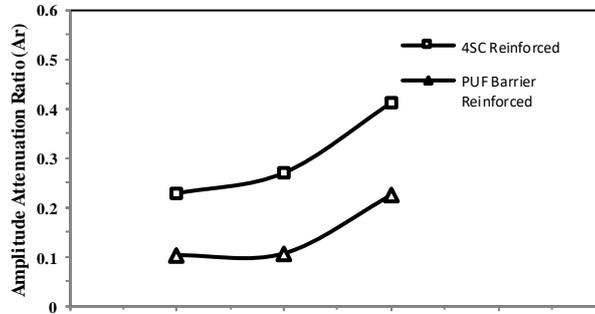
**Fig. 6.** Variation of Amplitude attenuation ratio curve observed under sub-sequential un-drained loading condition.
