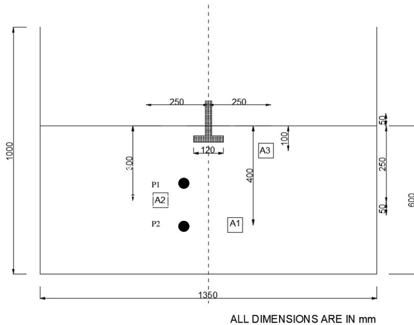
**Fig. 2.** Unreinforced model ground – Sectional view
