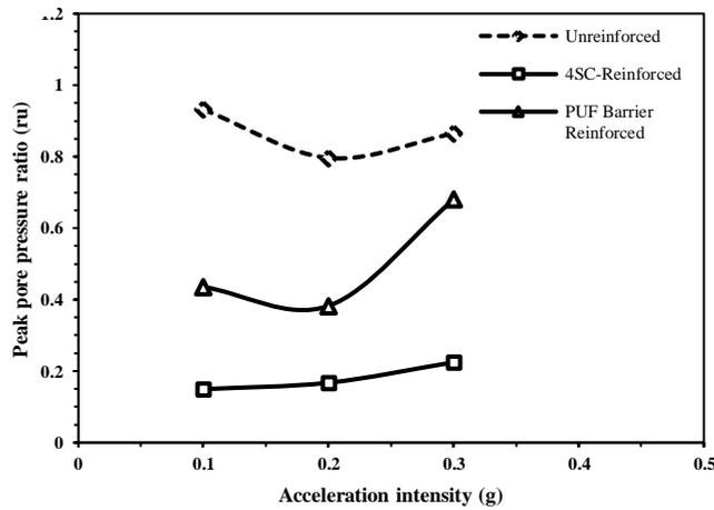
Fig. 7. Variation of peak pore pressure ratio observed under sub-sequential acceleration loading condition.
