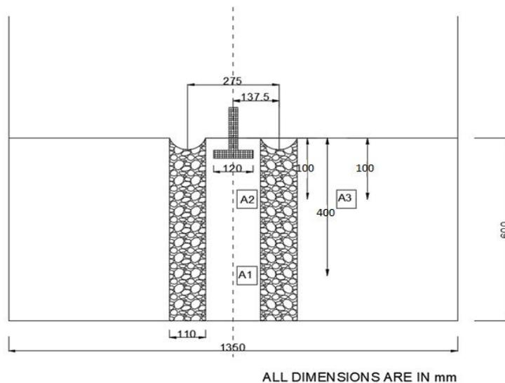
**Fig. 3.** Model ground reinforced with four stone columns – Sectional view
