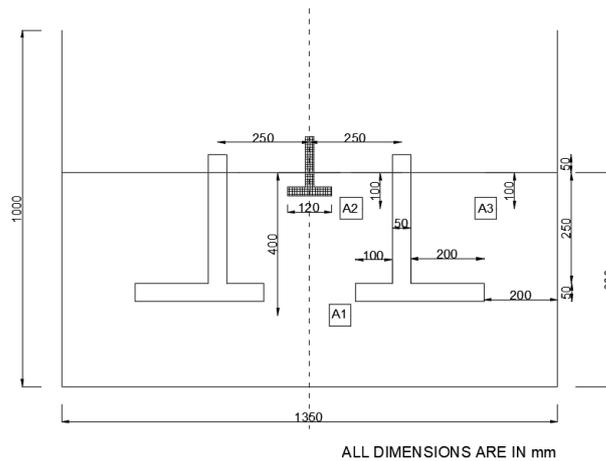
Fig. 4. PUF confined barrier reinforcement system – Sectional view
