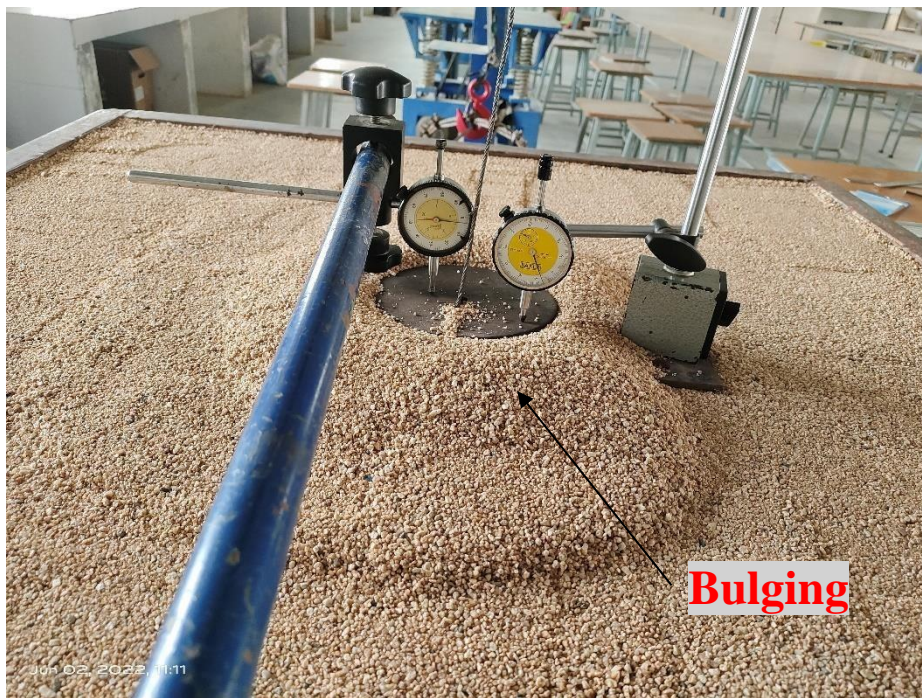
Fig. 3 A Photographic view of reinforced sand bed after failure.
