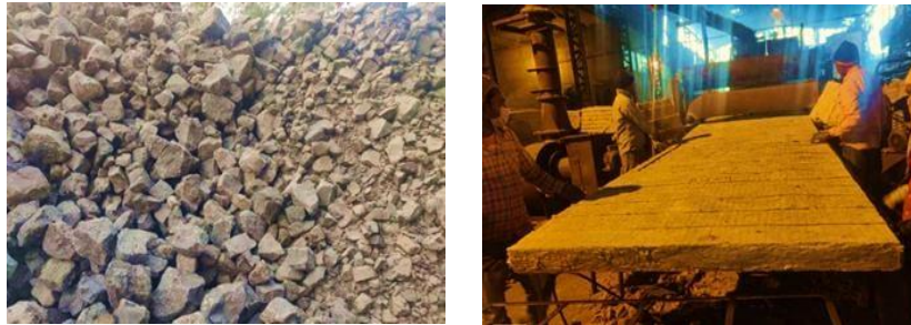
(a) (b) Fig 1. (a) Basalt material (b) Manufactured Rockwool Sample
