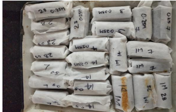
Fig. 2. Curing of specimens
