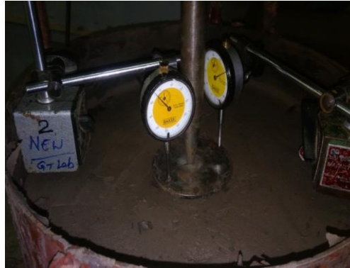
Fig.5. Dial gauges on loading plate
