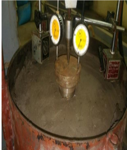
Fig.7. (1) Preparation of a stone column, (2) Loading plate placed on the stone column area, (3) Dial gauges was arranged on loading plate
