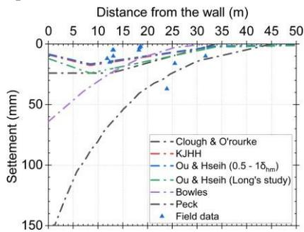
**Fig. 10.** Predicted vs observed settlements for mechanical slab
