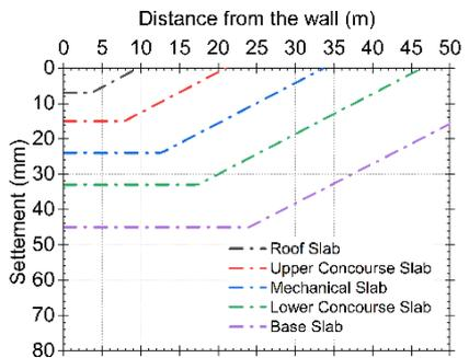
Fig. 7. Settlement predicted using Clough & O'Rourke (1990)
