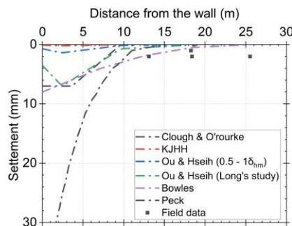
Fig. 8. Predicted vs observed settlements for Roof slab
