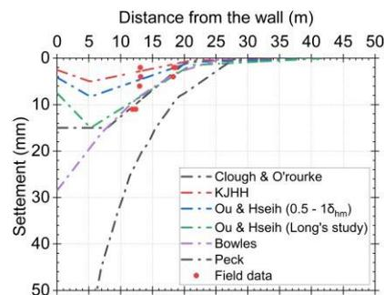
Fig. 9. Predicted vs observed settlements for Upper Concourse slab
