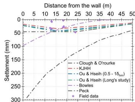
**Fig. 12.** Predicted vs observed settlements for base slab
