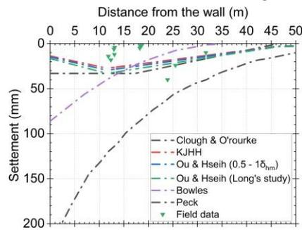
**Fig. 11.** Predicted vs observed settlements for lower concourse slab
