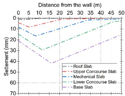
Fig. 5. Settlement predicted using Hsieh & Ou (1998) with  $0.5-1 \delta_{hm}$
