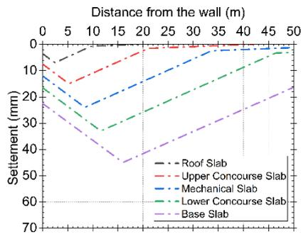
Fig. 4. Settlement predicted using Hsieh & Ou (1998) with Long's study
