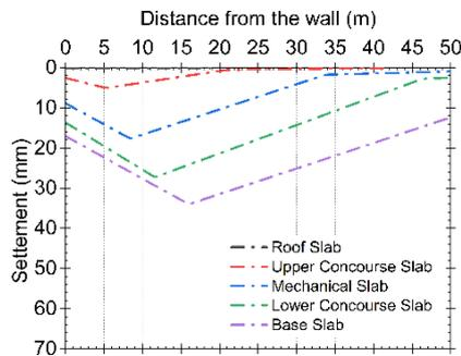
Fig. 6. Settlement predicted using Kung et al. (2007)
