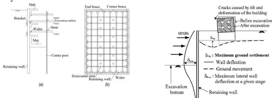
**Fig. 1.** Braced excavation method: (a) profile and (b) plan (c) Ground surface settlement induced by lateral wall movement.
