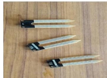
Fig. 2. Locations of the sensors in the model and the SEN0114 soil moisture sensor
