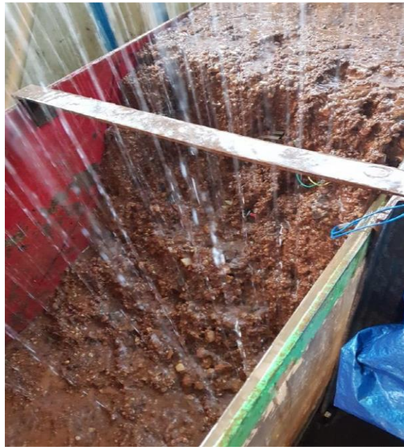
Fig. 4. Failure of 60° slope model
