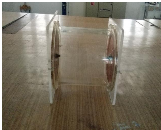
Fig. 2. Fabricated soil resistivity box
