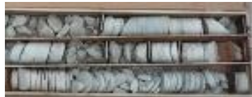
Fig. 2. Core dinking due to stress effect in Quartzite
