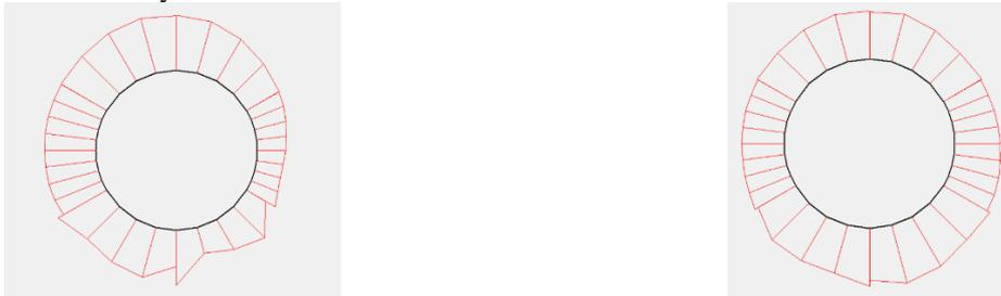
The extreme axial force experienced by tunnel 1 is  $62.58 \cdot 10^{-3}$  kN/m and that of tunnel 2 is  $73.57 \cdot 10^{-3}$  kN/m.
