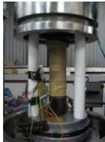
Fig. 3. Complete triaxial setup for UCS and triaxial testing (a) loading frame, (b) data accusation system
