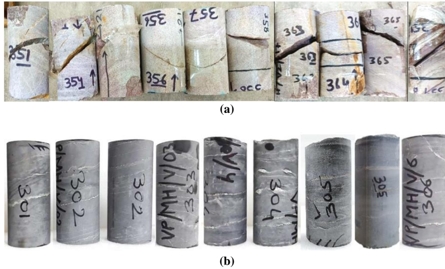
Fig. 1. Selected samples of (a) Open jointed Quartzite rock, (b) Tight jointed Slate rock
