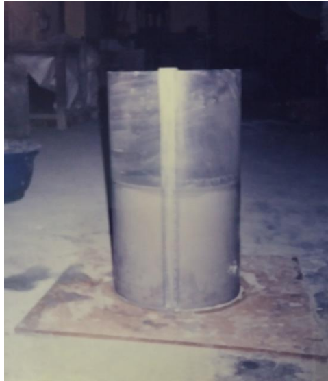
Fig. 1. Settling of Fly ash (Cylinder dia 298.5 mm)
