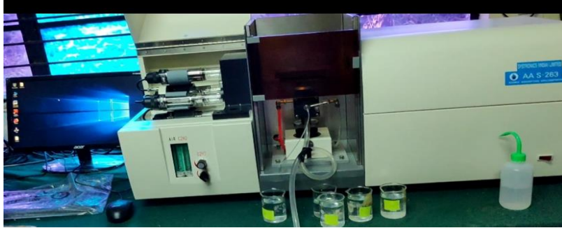
Fig. 1. Atomic absorption spectrometer (AAS) test setup
