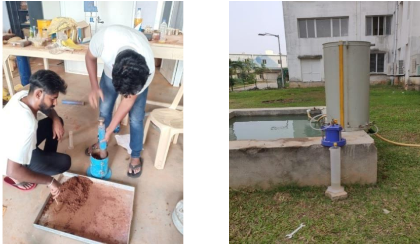
Fig 2. Compaction test and permeability test being conducted on the soil samples
