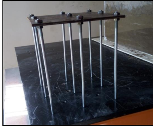
Fig. 5. Piled raft model
