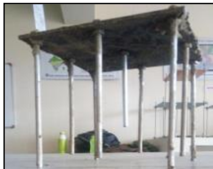
Fig. 7. various arrangement of pile
