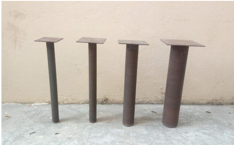
Fig. 1. Steel pipe piles
