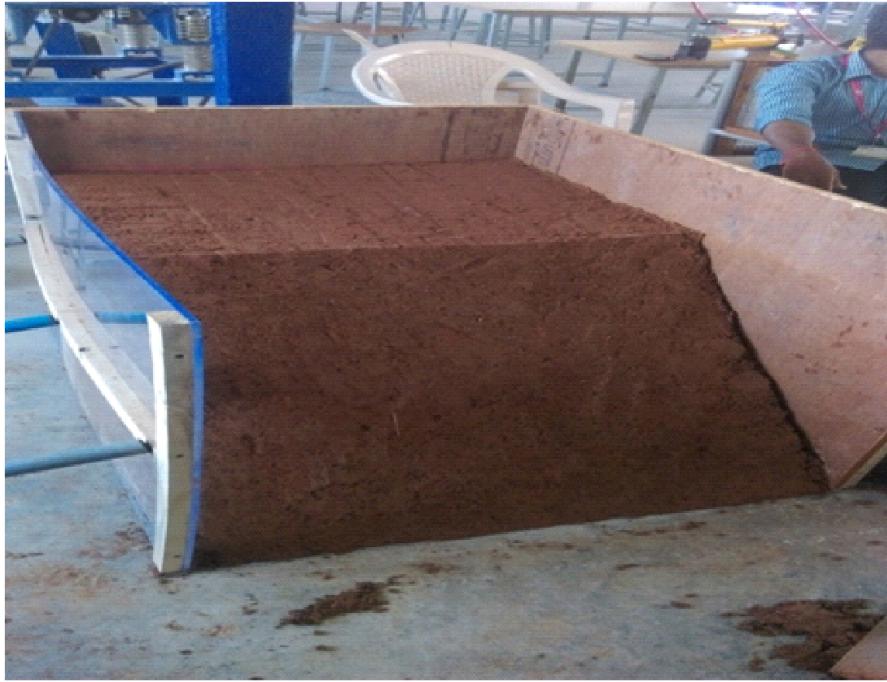
Fig. 1a. Embankment placed in the test tank with an angle of 45°
