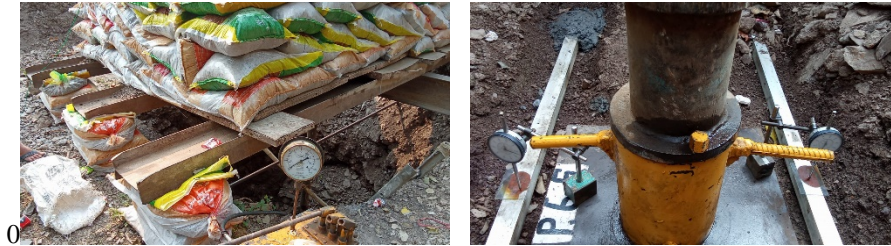
Fig. 10. Plate Load Test in progress
