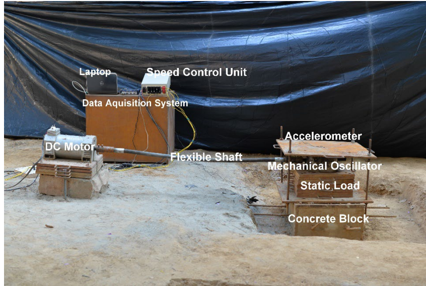
Fig. 1. Experimental Test Setup for Vertical Vibration
