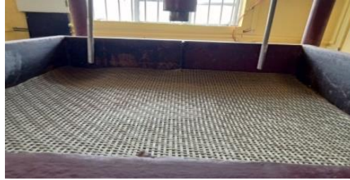
Fig. 5. Square aperture bamboo grid at required depth
