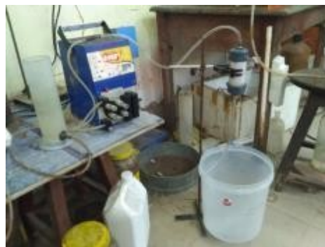
Fig. 2. MICP treatment process through peristaltic pump
