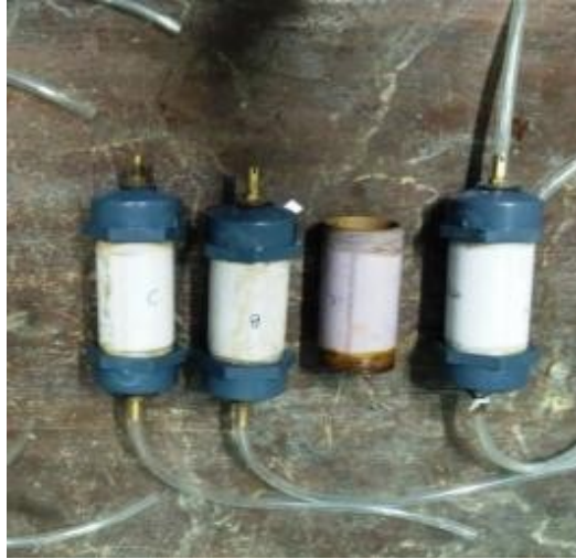
Fig. 1. PVC moulds for specimen preparation
