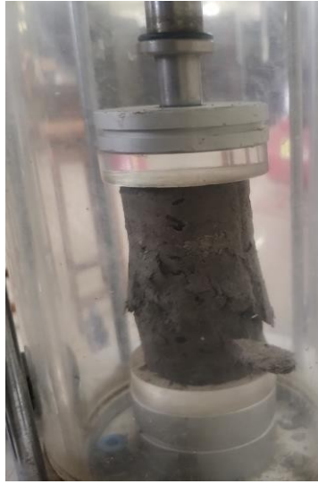
Fig. 6. MICP treated fly ash sample after UCS test
