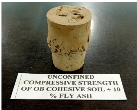
Fig. 02. UCS test on OB Sample
