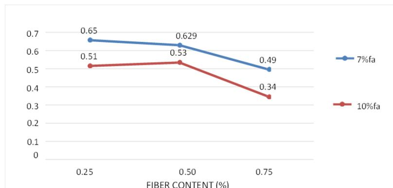
**Fig. 3.** Variation of Crack Width with Fiber Content
