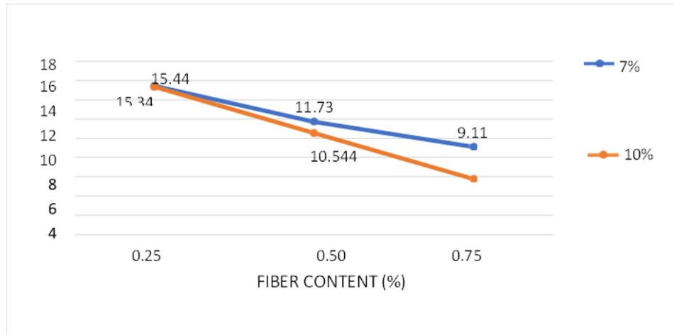
Fig. 4. Variation of Crack Length with Fiber Content
