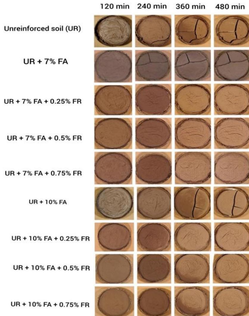
Fig. 2. Desiccation test results for every two hours
