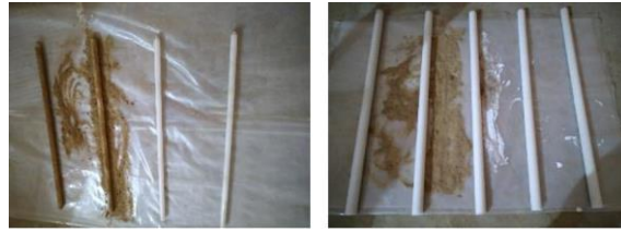
Fig. 2. Recycled plastic pins used as micropile of diameter 22 mm and 30 mm
