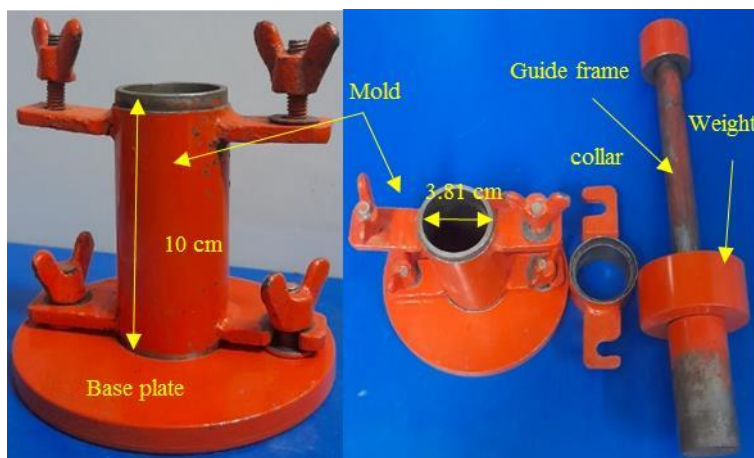
Fig. 1. Mini compaction test apparatus (Sridharan & Sivapullaiah, 2005).
