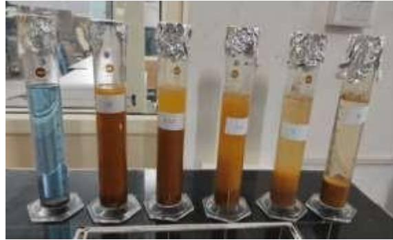
Fig. 1. Swelling of soil at different dosage of TerraZyme
