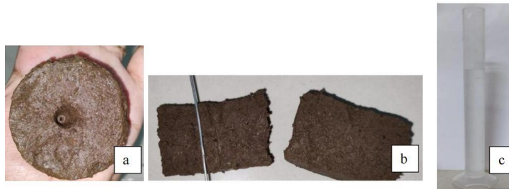
Fig. 11. (a and b) Size of hole and (c) clear effluent after 1.5% NS addition
