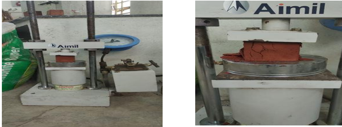
Fig.6: Compressive strength test
