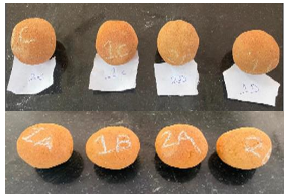
Fig. 4: Trial balls after burning
