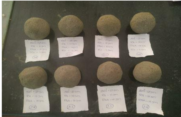
Fig. 3: Trial balls before burning
