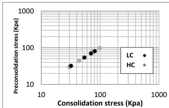
**Fig. 14.** Variation of Preconsolidation stress with consolidation stress (OMC)
