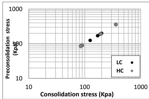
Fig. 5. Variation of Preconsolidation stress with consolidation stress (OMC)
