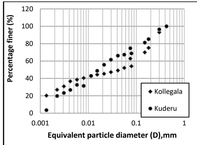
**Fig. 2.** Grain size distribution curves for Kollegala and Kuderu soils
