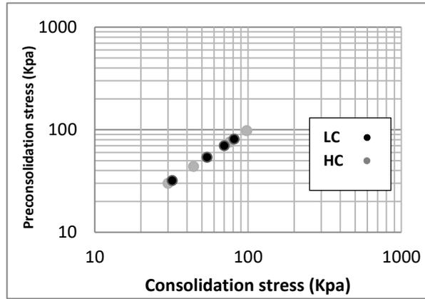
**Fig. 13.** Variation of Preconsolidation stress with consolidation stress (Dry side)
