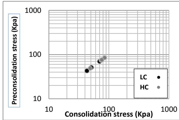
**Fig. 7.** Variation of Preconsolidation stress with consolidation stress (Dry Side)
