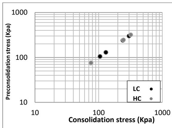
Fig. 12. Variation of Preconsolidation stress with consolidation stress (Wet side)
