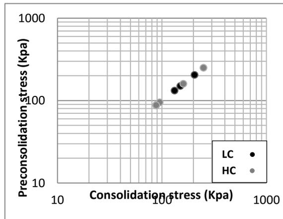
**Fig. 8.** Variation of Preconsolidation stress with consolidation stress (OMC)
