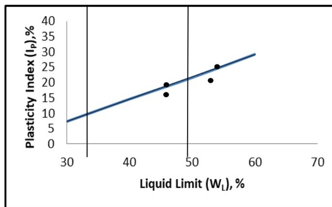
**Fig. 3.** Position of the soils under study on the plasticity chart
