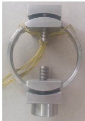
Fig. 1. View of proving ring, The fabricated ring used in the laboratory.
