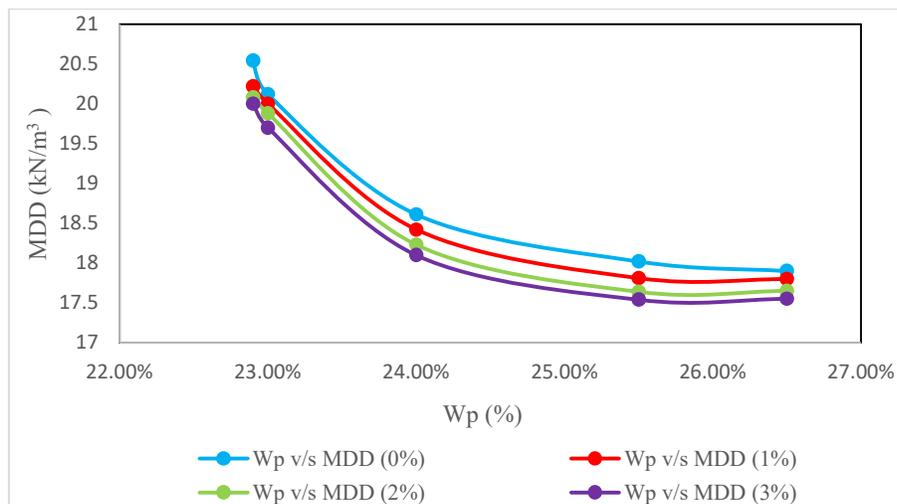
Fig. 6. Relation between MDD and plastic limit
