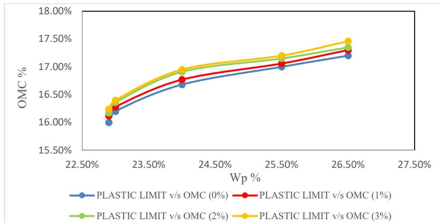
Fig. 5. Relation between OMC and plastic limit
