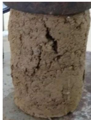
**Fig. 3.** Failure pattern of B30:Q70 sample
