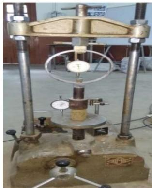
**Fig. 2.** UCS test setup.
