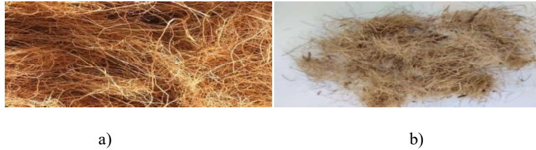
Fig.1. a) coir fiber, b) coir fiber of 20mm length
