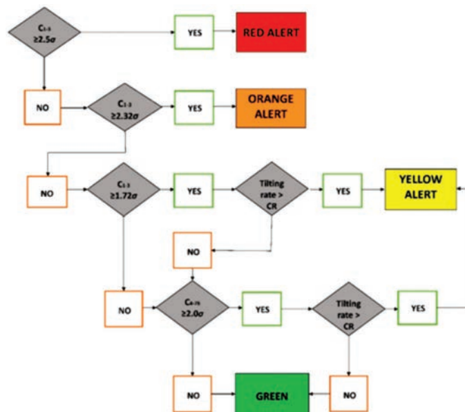
Figure 1: Decisional algorithm used for calibrating the combined SIGMA+tilt model for Kalimpong (Abraham et al., 2021a)
