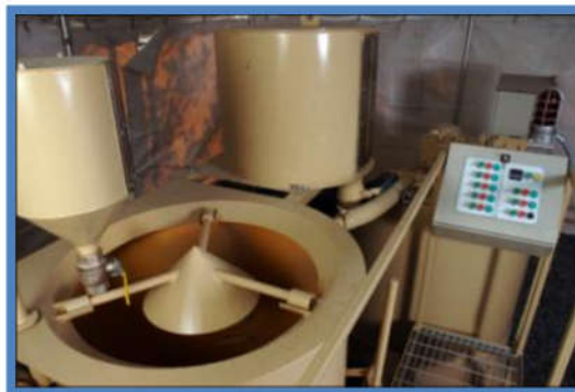
Figure 7.17. Gravity-feed admixture dispenser tanks re-filled via admixture pumps, with a 15-L polymer tank on the left and a 200-L bentonite slurry tank on the right with sight glasses for dosing. (Courtesy of Gannett Fleming)
