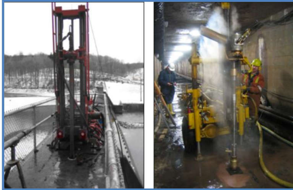
Figure 7.3. High-speed rotary drills for difficult access and confined spaces
