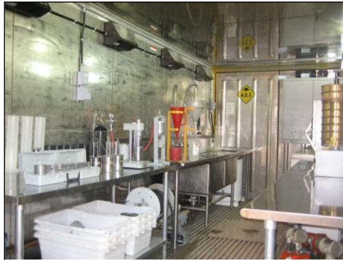
Figure 5.9. On-site quality control testing lab (Courtesy of Advanced Construction Techniques)
