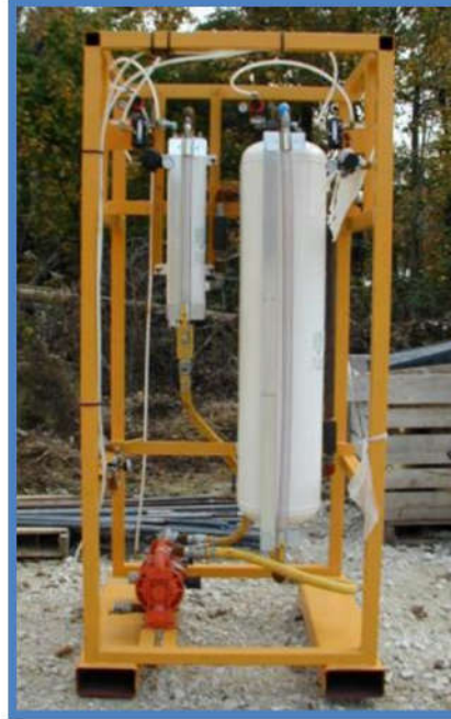
Figure 7.16. Pneumatic additive dispensers. (Courtesy of Advanced Construction Techniques)
