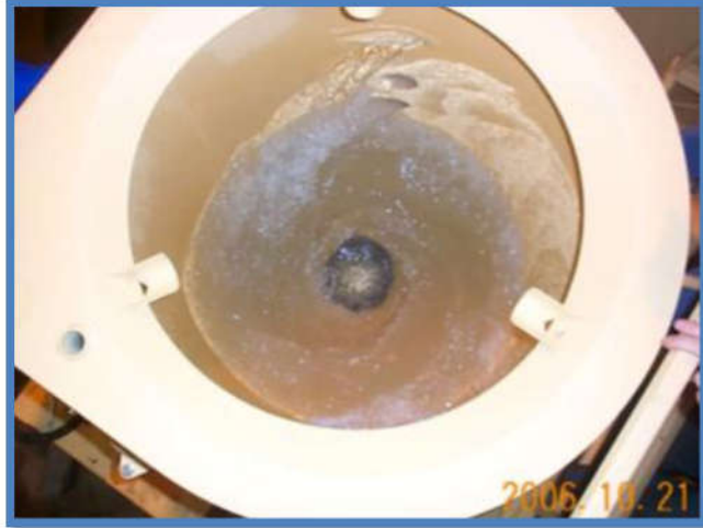
Figure 7.13. Vortex inside a high-shear mixer. (Courtesy of Gannett Fleming)
