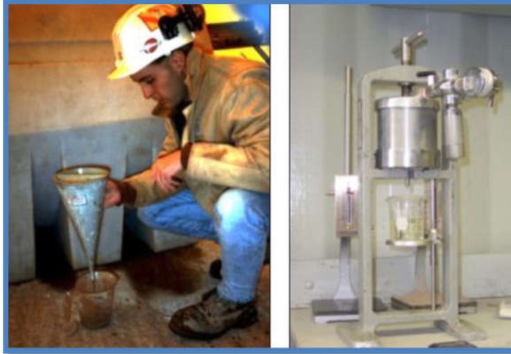
Figure 5.7. Testing for apparent viscosity and pressure filtration. (Courtesy of Gannett Fleming)
