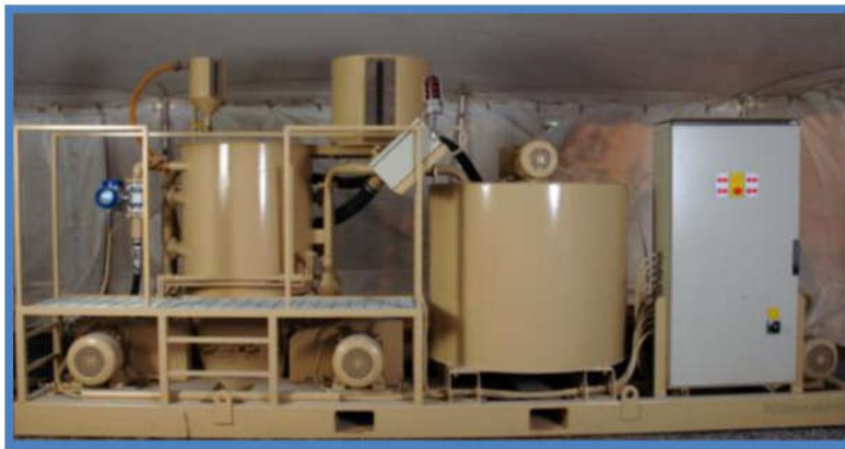
Figure 7.14. 500-L high-shear mixer with a 1,500-L agitator. (Courtesy of Gannett Fleming)
