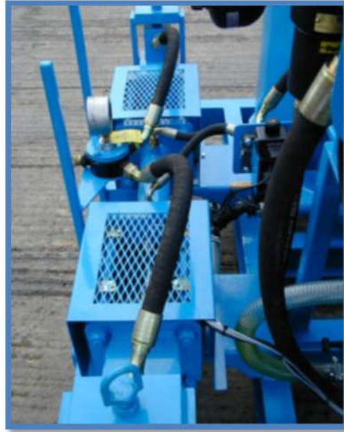
Figure 7.19. Piston pump with a reciprocating power source.(Courtesy of Gannett Fleming)
