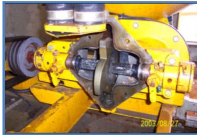
Figure 7.12. Rotor of a high-shear mixer with the mixer cover removed. (Courtesy of Advanced Construction Techniques)
