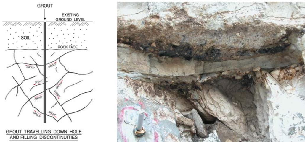
Figure 8: Depiction of Fissure Grouting and End Product
