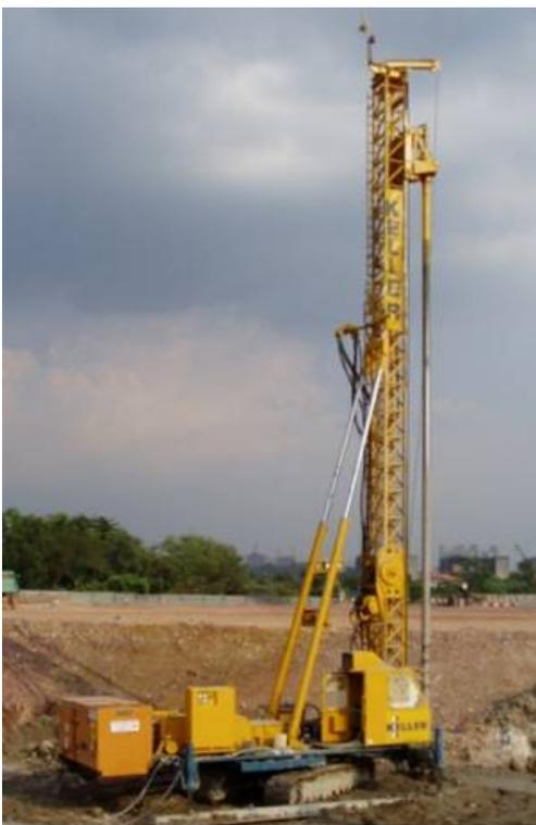
*Fig. 7."Wet" DSM rig*
