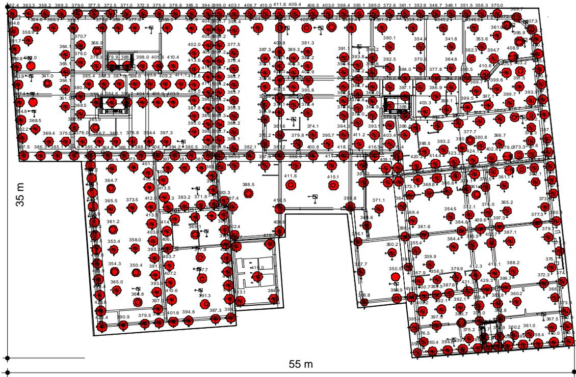
Figure 3. Arrangement of SM columns under the foundation slab of multistory building (Kielce, Poland).
