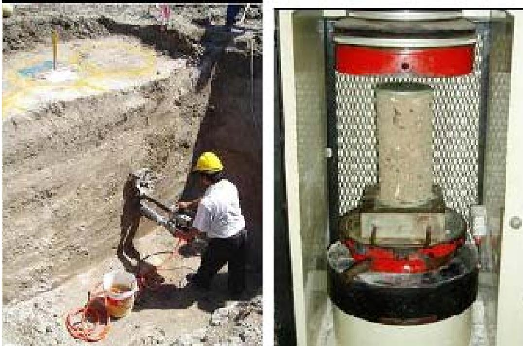
*Fig. 16 Horizontal coring and UCS testing*
