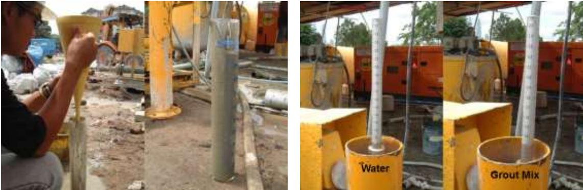
Figure 11: Marsh cone on Grout & Hydrometer test on grout and Water
