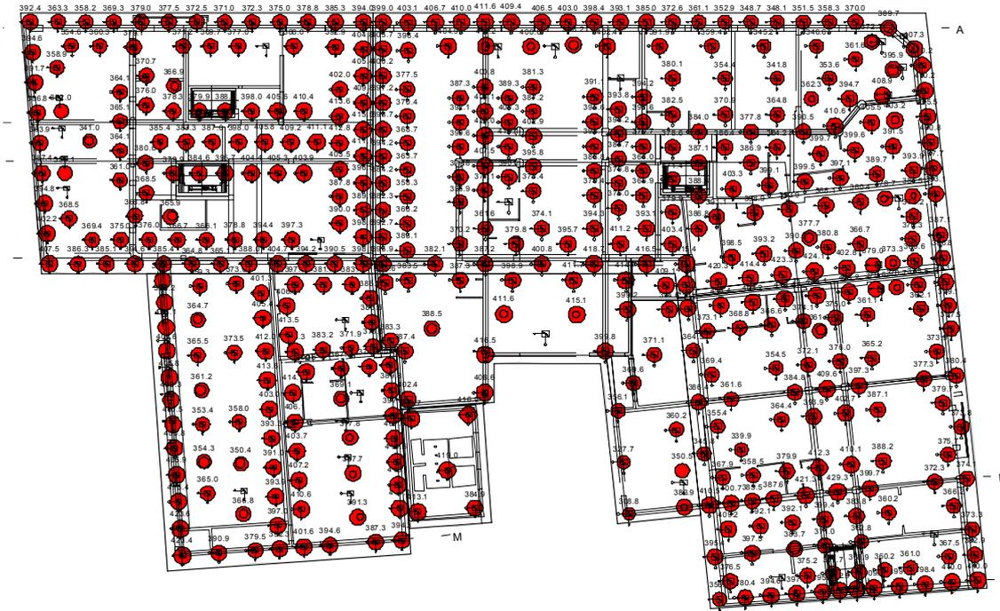
Fig. 5. Arrangement of DSM columns under the foundation slab (size of each circle indicates column load in kN)
