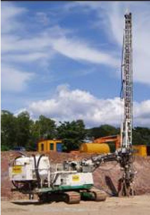
*Fig. 6."Dry" DSM rig*
