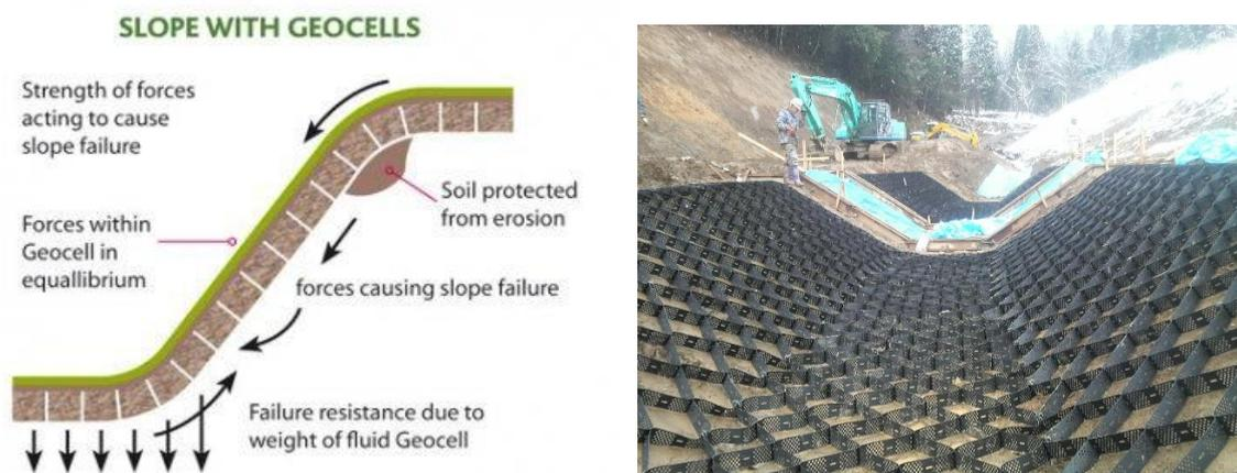
**Figure 35.** Schematic diagram and photograph of geocell erosion control system
