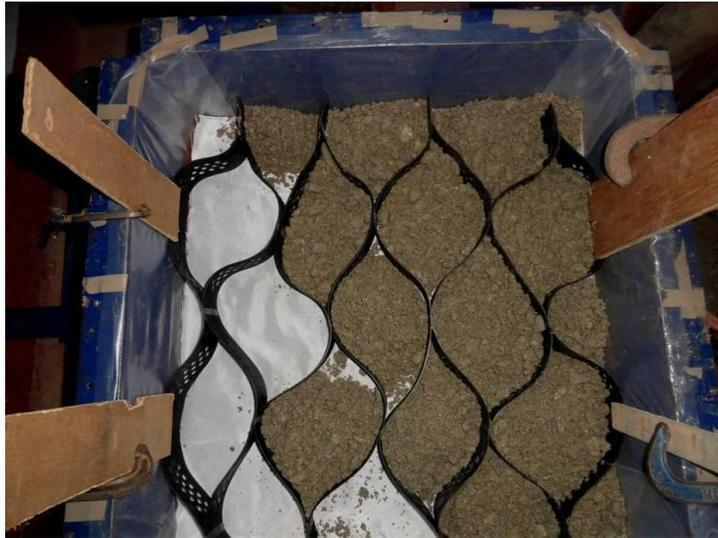
**Figure 26.** Photograph of aggregate being filled in geocell pockets
