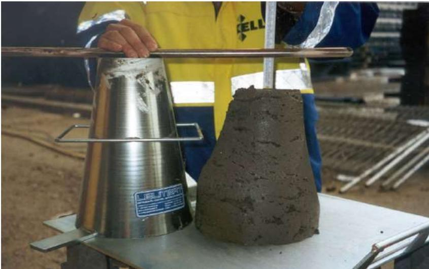
Figure 12: Slump cone test
