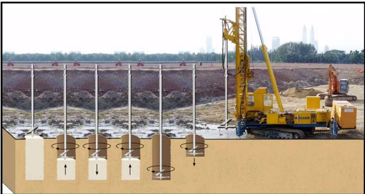
**Figure 7: Overall process in Wet DSM**
