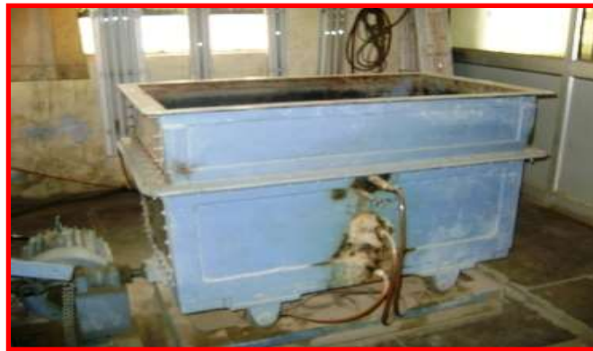
Fig. 1. Liquefaction Table used in the Experiments at IIT Roorkee
