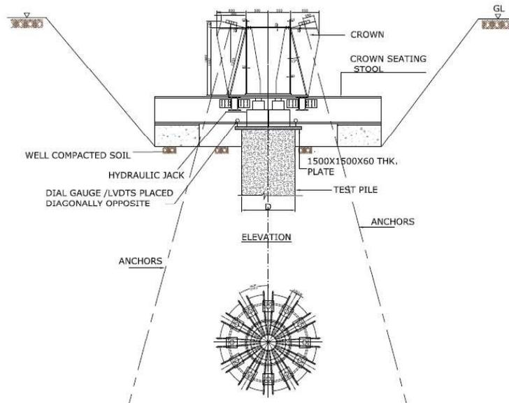
**Fig. 3.**Crown Girder Setup
